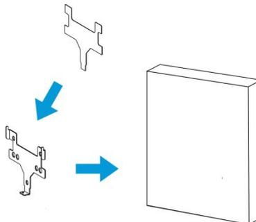
2. Put the device on the mounting bracket, then fix the bottom of the device to the bracket with the theft-detering screw.
