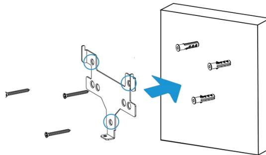
2. Put the device on the mounting bracket, then fix the bottom of the device to the bracket with a fixing screw.
